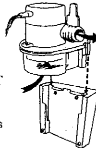
Pump is easily removed by pushing tab and sliding pump assembly up and out of bracket.
